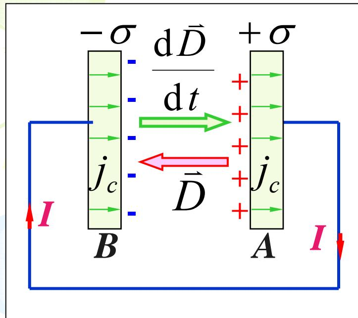
$$I_c = \frac{dq}{dt} = \frac{d(S\sigma)}{dt} = S \frac{d\sigma}{dt}$$
