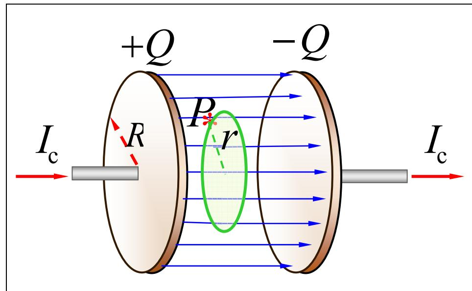
$$\because D = \sigma \quad \therefore \Psi = \frac{r^2}{R^2} Q \quad I_d = \frac{d\Psi}{dt} = \frac{r^2}{R^2} \frac{dQ}{dt}$$
